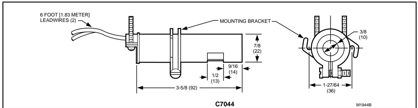
Fig. 3. Installation dimensions of C7044A in in. (mm).
