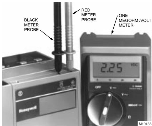
**Fig. 9. Measuring voltage flame signal with 7800 SERIES controls.**
